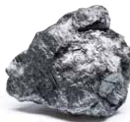
Ore from Sri Lanka: This ore features a special structure and a high graphite content of up to 99%
