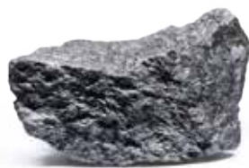
Ore from Kropfmühl: Graphite content of up to 30% in the ore
